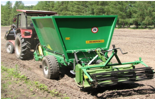
Fig. 1. SRS Fertilizer dispenser at work in nursery
