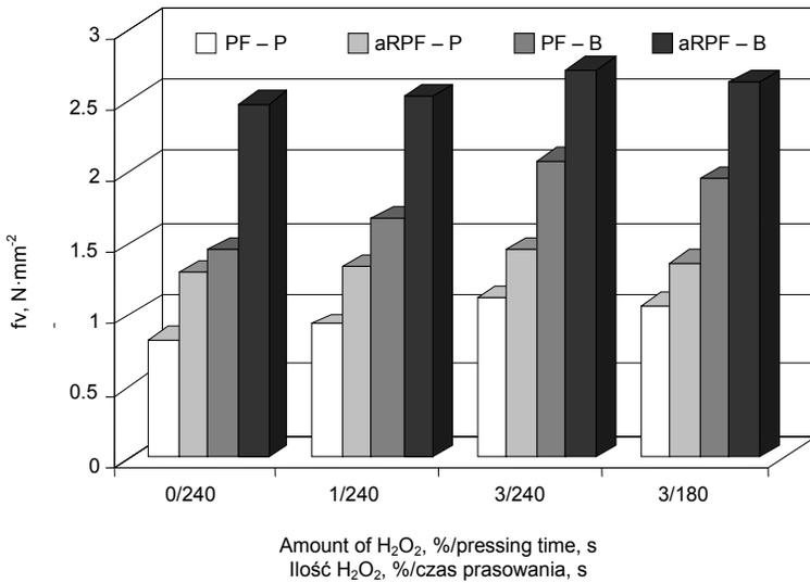
Fig. 2. Shear strength of plywood manufactured with modified PF resin after boiling test: P – pine, B – beech
