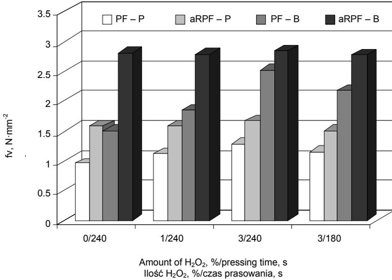
Fig. 1. Shear strength of plywood manufactured with modified PF resin after soaking in cold water: P – pine, B – beech
