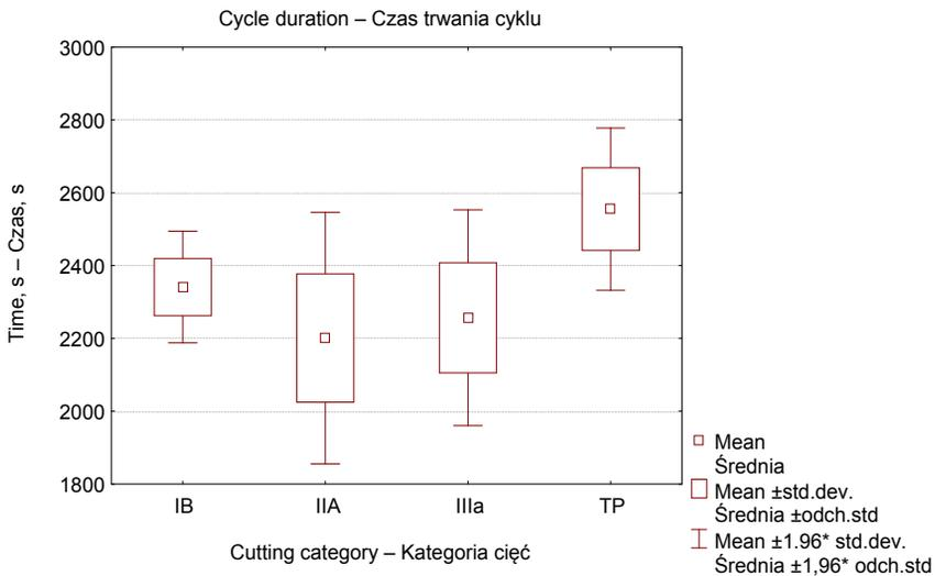
Fig. 1. Diagram of basic working cycle duration statistics while chipping wood representing various cutting categories
