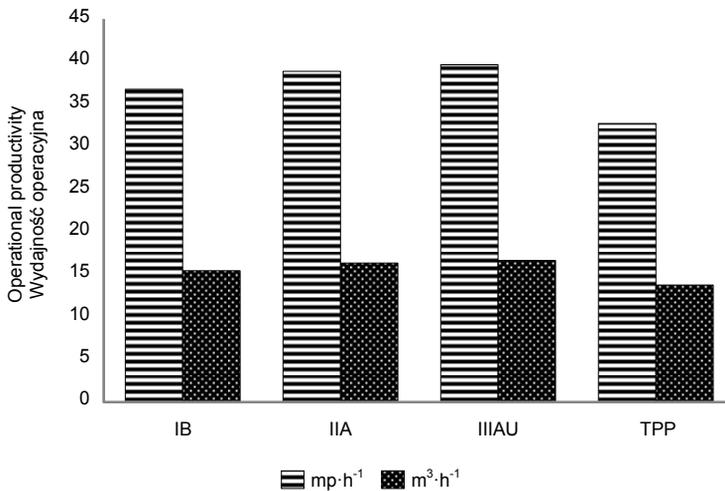
Fig. 2. Operational productivity of a working cycle of chipping logging residues
