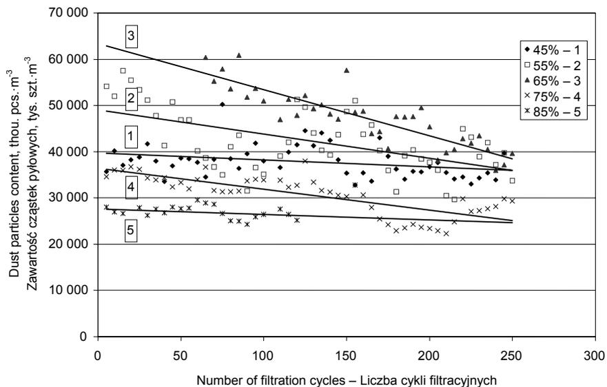
Fig. 2. Number of dust particles in air cleaned on hydrophobically appreted unwoven fabric
