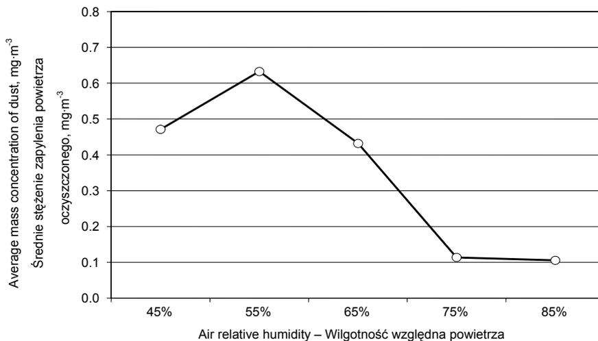
Fig. 5. Average dust concentration in cleaned air
