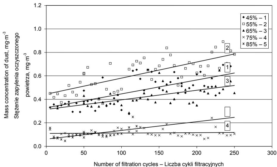
Fig. 4. Mass concentration of dust in air cleaned on hydrophobically appred unwoven fabric
