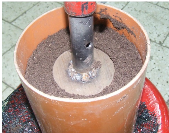
Fig. 2. Process of exerting the pressure on soil with use of the stamp
