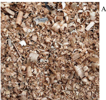
Fig. 2. Waste particles of natural oak wood A and thermally modified oak wood B resulted from operation 2
